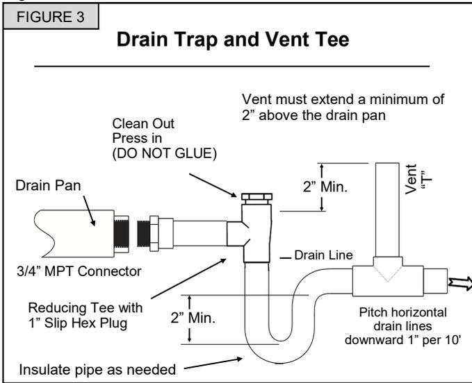
Route drain line so that it does not interfere with accessibility to the coil, air handling system or filter and will not be exposed to freezing temperatures.
