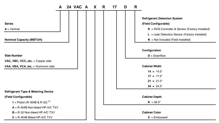
[1] R-454B Piston factory installed to match the nominal BTU rating of the coil.
